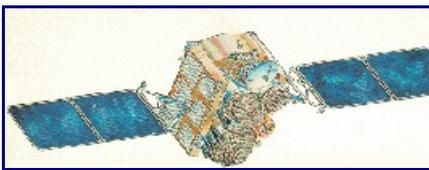
The DSCS III system is built with single- and multiple-beam antennas that provide more flexible coverage than its predecessors. Phase III satellites bring more capacity while providing greater assured communications through improved ability to resist jamming. Antenna design for DSCS III allows
