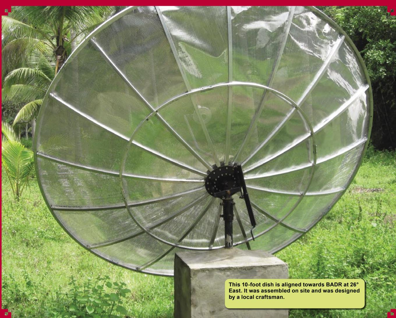
This 10-foot dish is aligned towards BADR at 26° East. It was assembled on site and was designed by a local craftsman.
