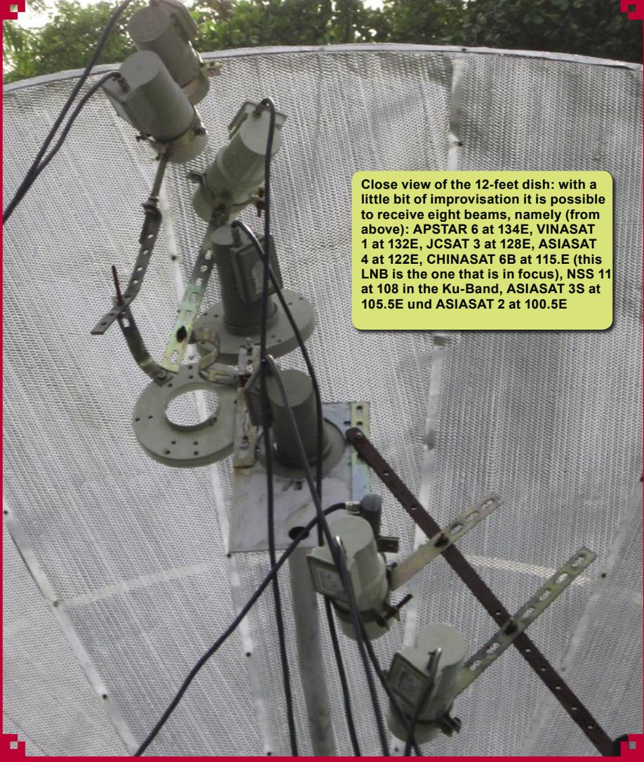
Close view of the 12-foot dish: with a little bit of improvisation it is possible to receive eight beams, namely (from above): APSTAR 6 at 134E, VINASAT 1 at 132E, JCSAT 3 at 128E, ASIASAT 4 at 122E, CHINASAT 6B at 115.E (this LNB is the one that is in focus), NSS 11 at 108 in the Ku-Band, ASIASAT 3S at 105.5E und ASIASAT 2 at 100.5E
